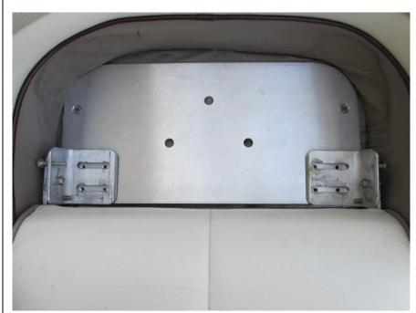
6. Reinstall the bolster hinges onto the repair plate
