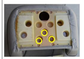
There are usually 3 philips head screws attaching the seat cushion to the seat assembly.
