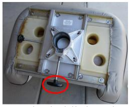
Unscrew the red circled knob. Once loose, you will be able to lift the seat off of the pedestal.
