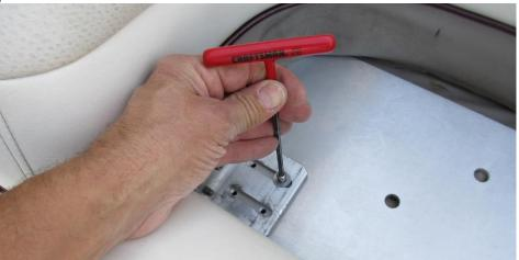
Using the 3 new longer screws provided, reinstall the cushion to the seat.
