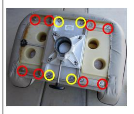
Remove the bolts circled in red holding the slide mechanism to the seat frame. You do not need to remove the bolts circled in yellow.
