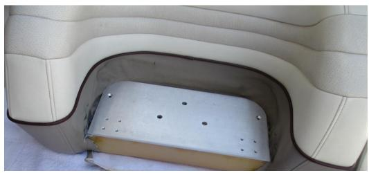
Place the plate on the seat pan. Make sure the counter sink side of the holes are facing UP (towards the cushion). Insert the assembly plugs into the large molded holes with the plastic part upwards.
