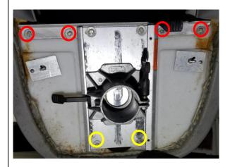
Remove the bolts holding the slide mechanism to the seat frame. NOTE: depending on the bolt arrangement, you may need to remove the entire upper bracket (4 red bolts) instead of the upper 2 yellow bolts
