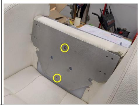
Go back and finish tighten the screws holding the lower assembly to the seat pan
