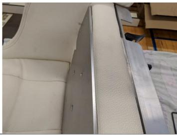
Using the original screws, reinstall the bolster hinges to the upper repair plate.
