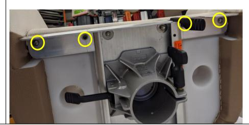
At this stage, the machined assembly installation is complete. There should be no play between assembly and the seat pan. If the screws are tightened and there is play between the seat pan and the structural assembly, then shims may need to be added to prevent relative motion between the seat pan and the structural assembly. Please contact <a href="slideruleracer@gmail.com">slideruleracer@gmail.com</a> for assistance.
