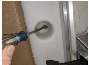
16. Reinstall the seat onto the pedestal
