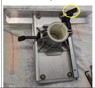
The lower assembly will be secured to the seat pan only via the threaded inserts that the OEM angle trim bar attaches to. If any of these inserts are damaged, it is OK – mostly, these screws are only needed to hold the assembly in place during the attachment of the top plate.
