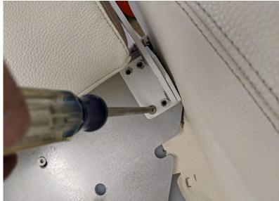
Using the 2 new longer stainless steel wood screws provided, reinstall the cushion to the seat. Reuse the original washers.
