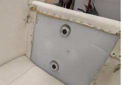
Align the upper plate into position as shown, making sure the countersink holes are facing up (out). Thread the 2 ½" Flathead screws through the upper plate into the standoffs. Get both screws started before tightening completely. While tightening, make sure the upper frame is centered in the seat and the front edge is aligned to the seat upholstery – adjust the position of the lower assembly if needed.
