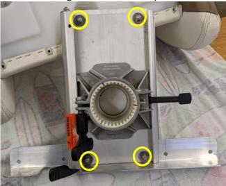
7. Fasten the Seat sliding frame to the lower plate
