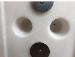
If necessary, use a fuel cap key while you tighten the %-20 stainless hex screws from above – most of the time the plug locks securely into the seat pan without the need for the fuel key.
