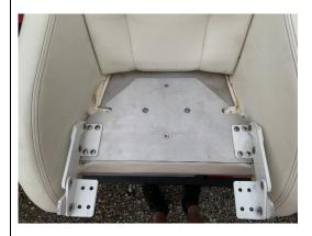
Place the plate on the seat pan. Make sure the counter sink side of the holes are facing UP (towards the cushion). Insert the assembly plugs into the large molded holes with the plastic part upwards. (plugs in photo below are older style)
