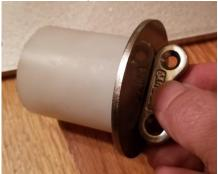
Make sure that the plugs are fully bottomed in the hole and that the stainless disc is pressed against the plastic seat base.
