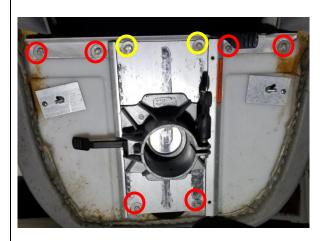
Remove the bolts circled in red holding the slide mechanism to the seat frame. You should not need to remove the bolts circled in yellow.
