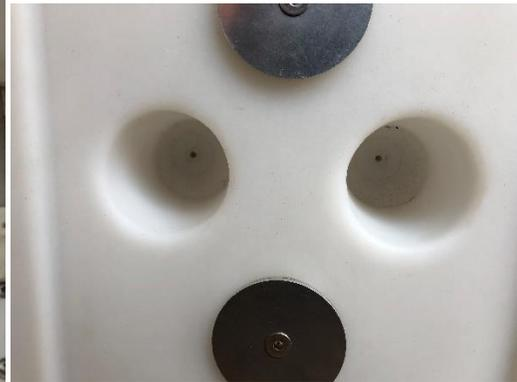
Use a fuel cap key or the included plastic key to hold the plug in place while you tighten the ¼-20 stainless Philips screws from above.
