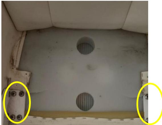
With the cushion removed, you now have access to the 8 screws holding the 2 bolster hinges to the molded seat pan.
